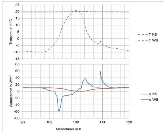
Fig. 9: Measurement values of temperature and heat flux for the material EPS 1 with a moisture content of 1,7 Vol-%
