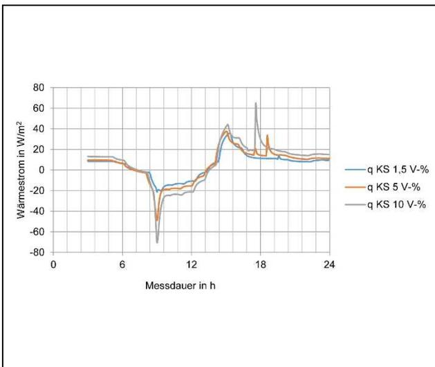
Fig. 10: Measurement values of heat flux for the material PUR with a moisture content of 1,5 Vol-%, 5 Vol-% and 10 Vol-%
