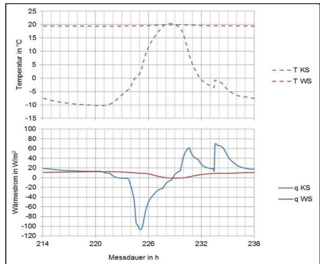
Fig. 11: Measurement values of temperature and heat flux for the material MW with a moisture content of 1,5 Vol-%.
