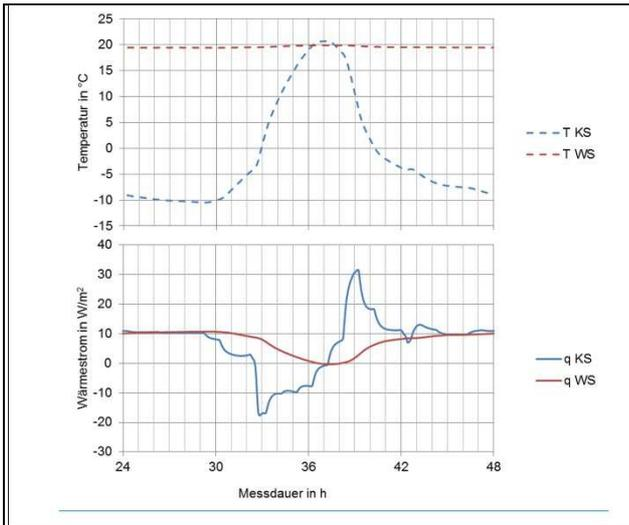
Fig. 8: Measurement values of temperature and heat flux for the material EPS 2 with a moisture content of 0,005 Vol-% (air-dry)
