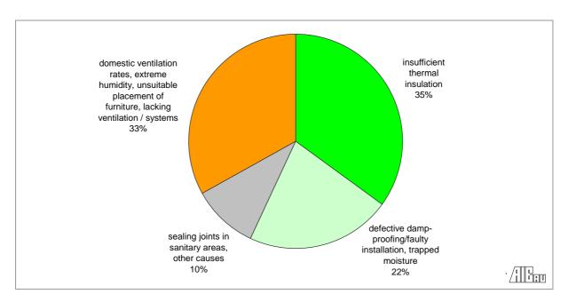
Figure 1: Causes of mould-related damage in highly insulated buildings (based on the description of 145 cases by publicly appointed and certified experts)
