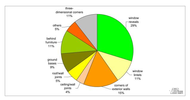
Figure 3: Location of ventilation-related mould damage in rooms (based on the description of 47 cases by publicly appointed and certified experts; multiple references possible)
