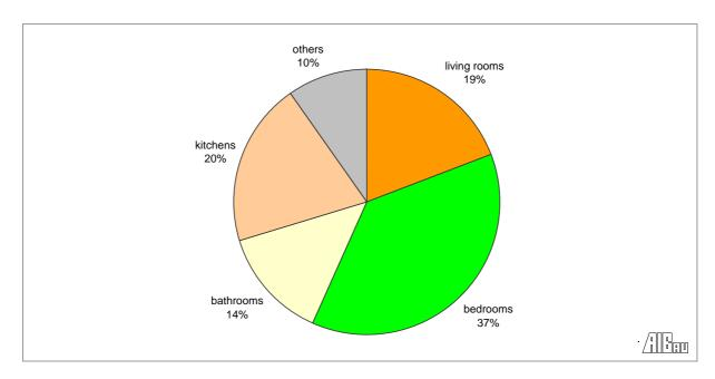
Figure 2: Occurrence of mould-related damage in various types of rooms (based on the description of 154 cases by publicly appointed and certified experts; multiple references possible)
