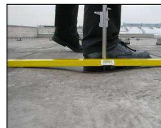
Measuring distortion under typical stress
